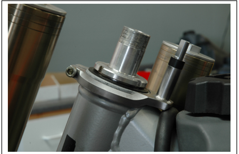
Here is the frame bracket installed, with the full circumference of the ring biting the head tube, also clearing the Triple clamp nuts.
