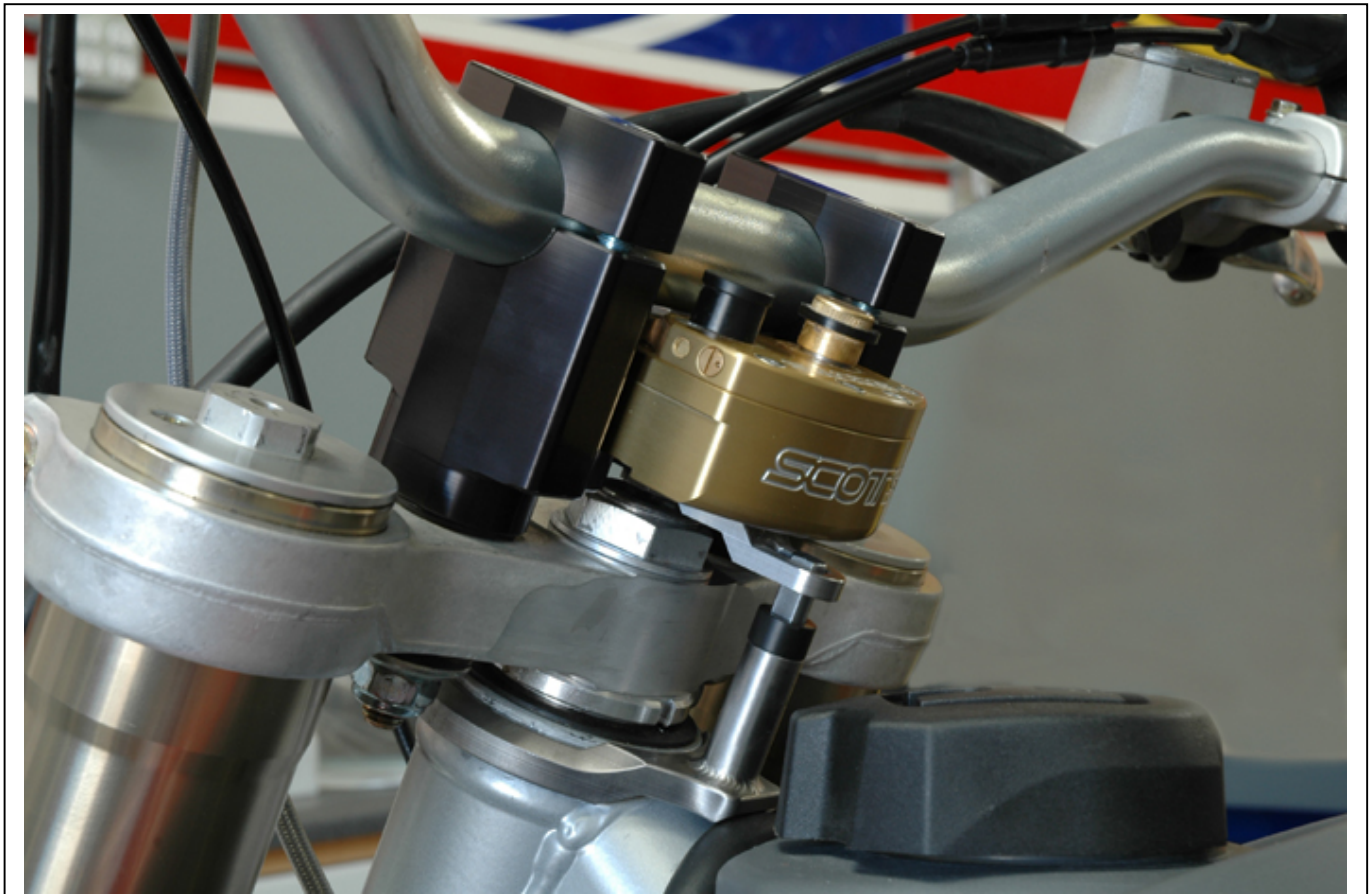
The Black Sub mount in this photo is only to help pronounce the part for the photo and installation ease. The actual Scott's Sub Mount is Titanium in color. This depicts the general mounting procedure.
