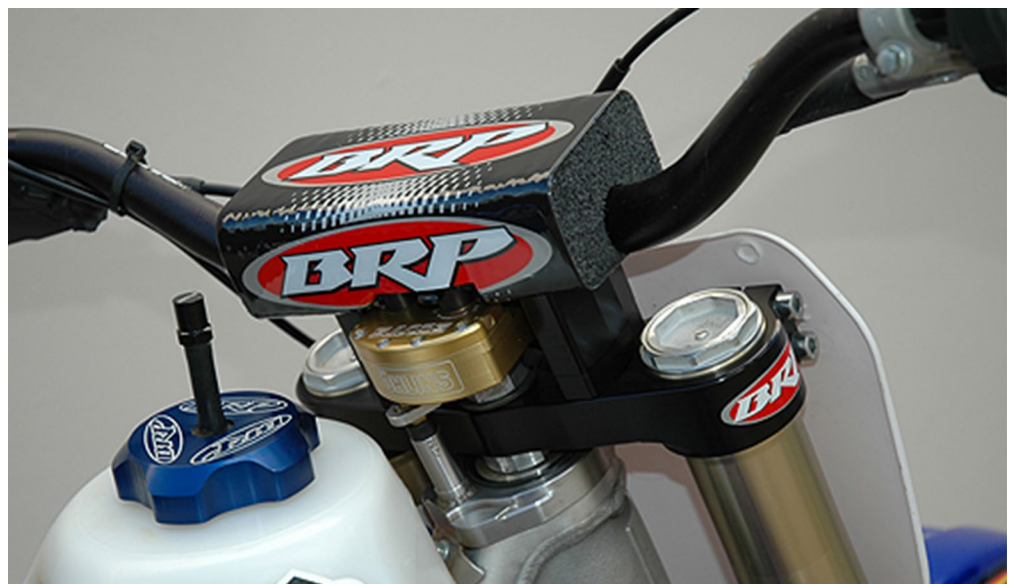
SUB mount installed with BRP clamps.
