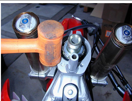
Tap, then tighten, tap and tighten until the bracket is down and securely flush
