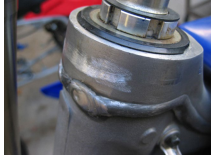
After bump is removed
