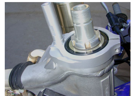
Frame bracket installed with the tower aligned straight on the backbone.
