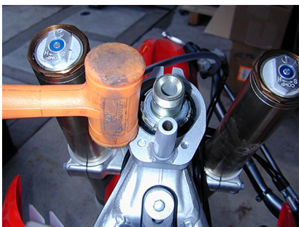
Tap, then tighten, tap and tighten until the bracket is down and securely flush
