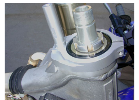
Frame bracket installed with the tower aligned straight on the backbone.
