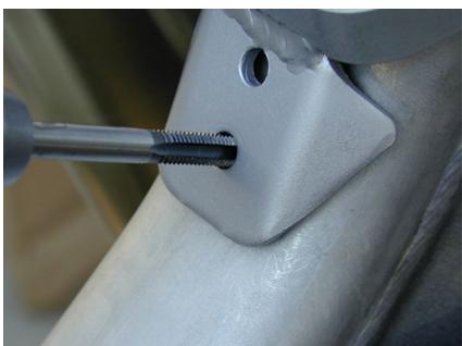
Drilling and tapping one hole at a time. Keep the drill and tap perpendicular to the bracket tab surface.
