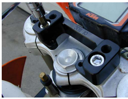
Bolt the Sub mount to stock triple clamp
