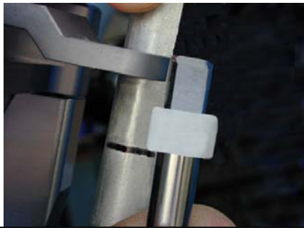
Marking where to cut the tower
