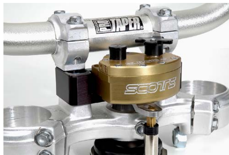
Bolt the stock barclamp to the Sub mount using the stock Allen bolts.
