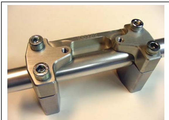
Mark and cut the tower so the flats are in the middle of the linkarm.
