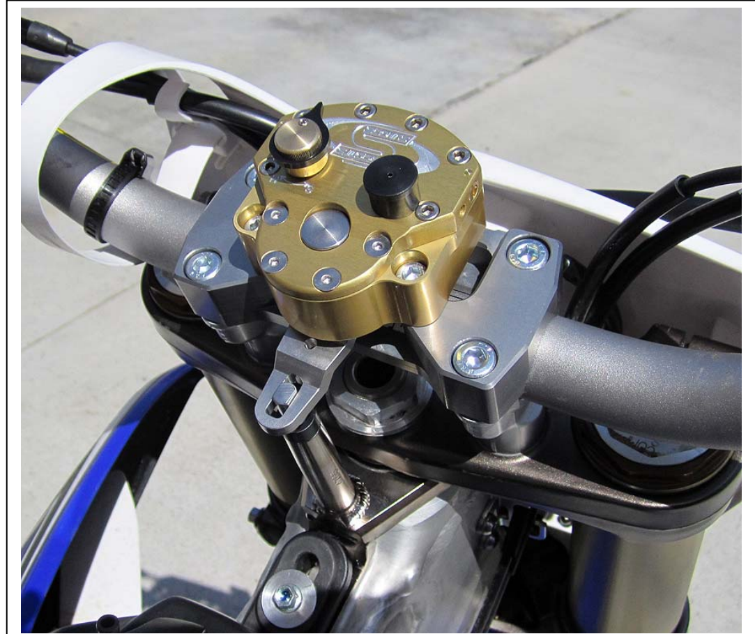
If the frame bracket tab is too low or too high do not try to bend it. Shim it or file the aluminum frame lug a little.
