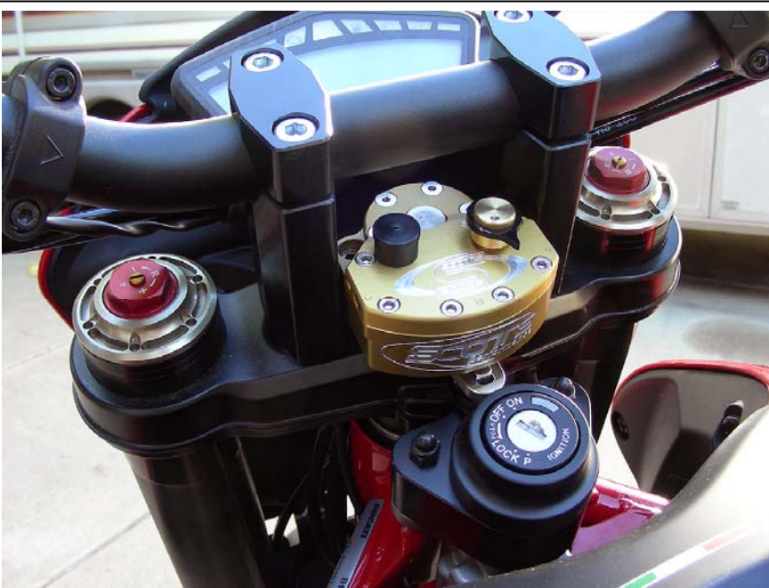
This shows the correct tower pin height
