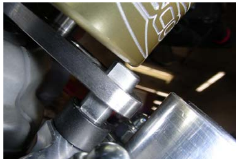
This shows the incorrect tower pin height.
