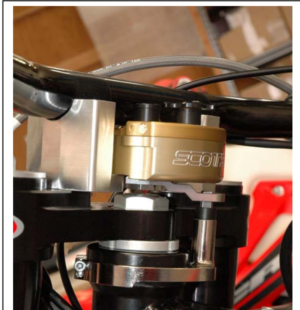
Be sure the tower pin is positioned as shown above and is not touching the bottom of the stabilizer body
