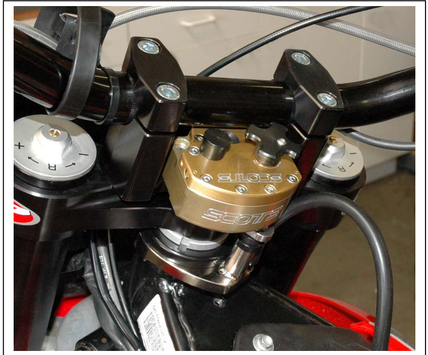
Be sure the tower pin is positioned as shown above and is not touching the bottom of the stabilizer body
