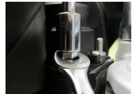
Remove the studs using 2 wrenches
