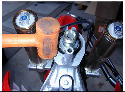
Tap bracket down until securely flush
