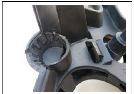
File the inside of both plastic bolt covers so its fits to your liking
