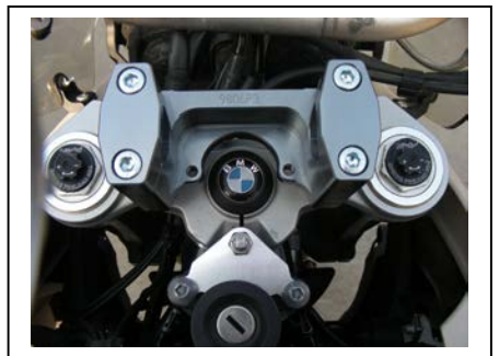
Sub mount installed correctly
