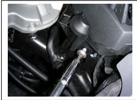
Remove the plastic torx key bolts
