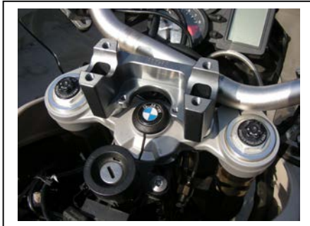
Lay bars forward out of the way & install Sub mount as shown
