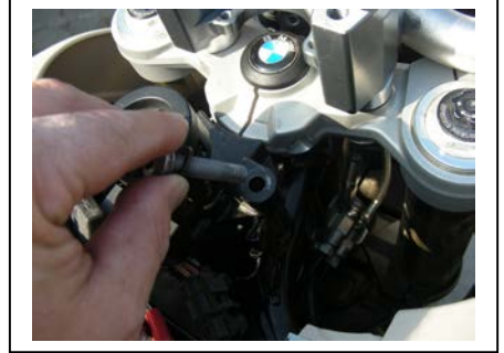
Stock key switch bolts are Torx remove and install frame bracket
