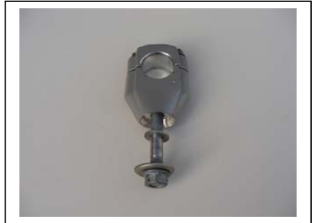
Remove the stock lower bar mounts
