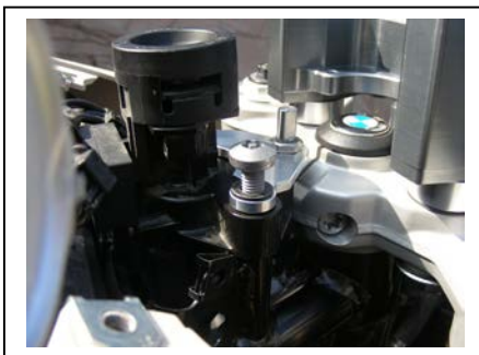
Frame bracket mounts as shown under the stock key mount bolts
