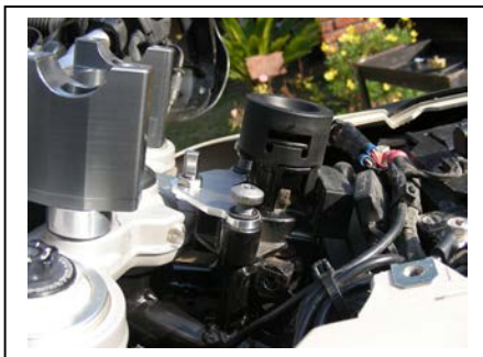
Side view of Sub & Frame bracket Spacers go under sub mount
