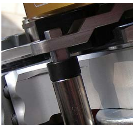
This shows the correct tower pin height for rubber mounted bars, with the tower pin 2mm above the top of the link arm.
