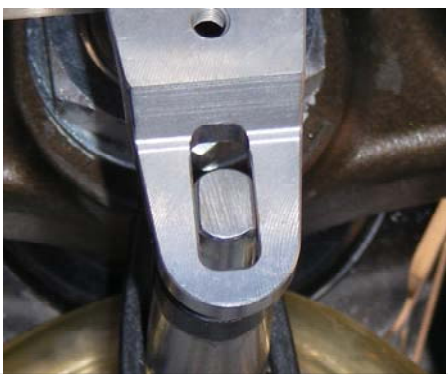
Try to center the pin in the linkarm slot, use welding rod on each side to
