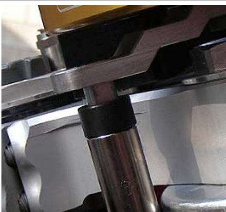
This shows the correct tower pin height for solid mounted bars, flush with the top of the link arm.
