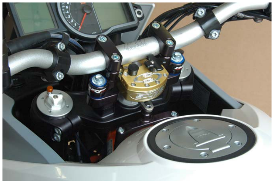
Tower Bridge installed correctly. Tower pin should be centered in link-arm when stabilizer is installed.
