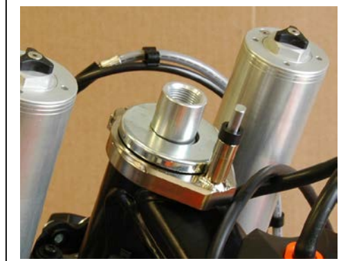
WRONG.... NOT FLUSH
