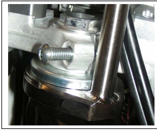
A special Low Profile pinch bolt is provided ONLY in kits that require additional clearance.
