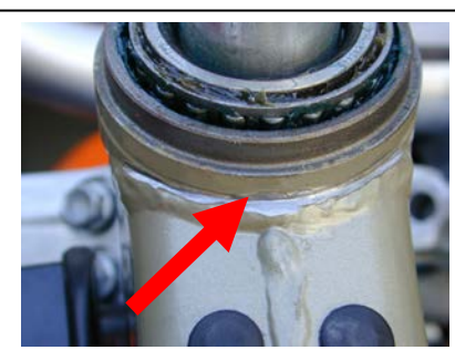
File any welds so the groove shows all the way around.
