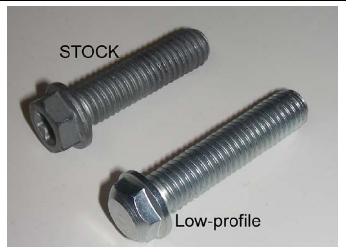
Shown here is the stock and new low profile bolt for the triple clamp pinch bolt on bikes with little or no clearance.
