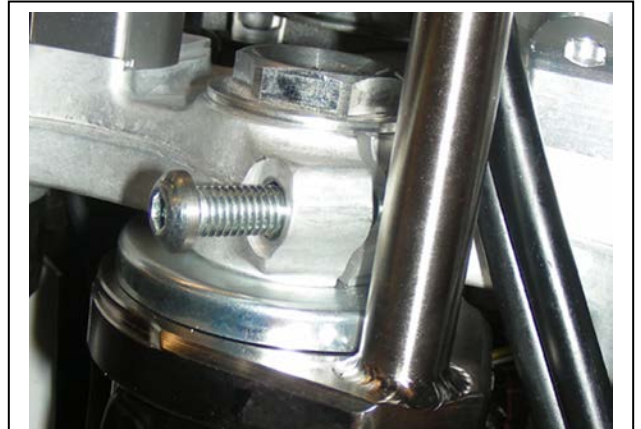
Install the special low profile bolt to gain more clearance as the triple clamp swings past the tower.
