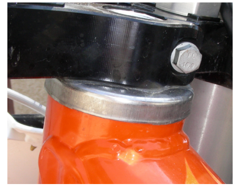
Red arrow shows clamping surface. Blue arrows show where to file welds, if necessary. Some bikes require no filing.
