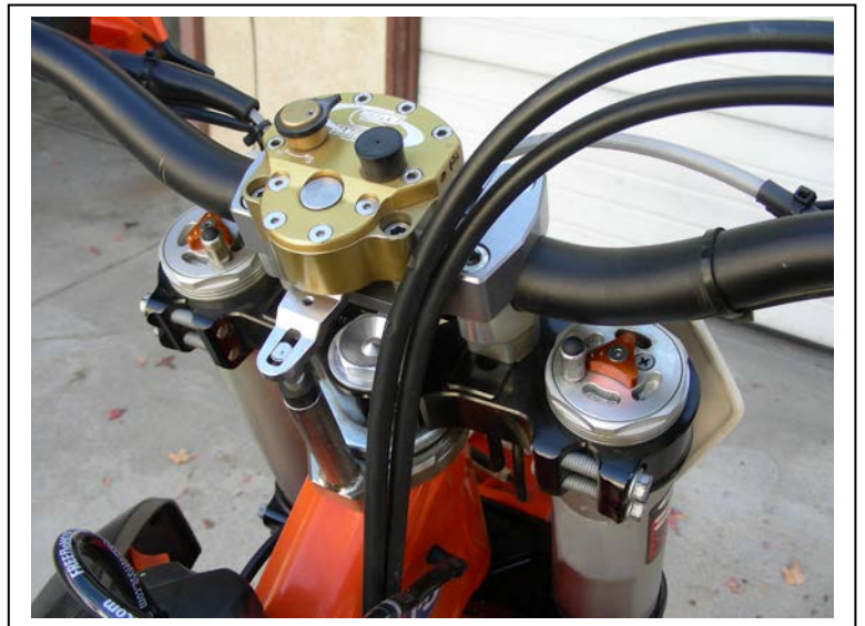
Install the special low profile bolt to gain more clearance as the triple clamp swings past the tower.
