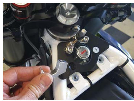
Move the top plate around until it's centered and up against the head tube
