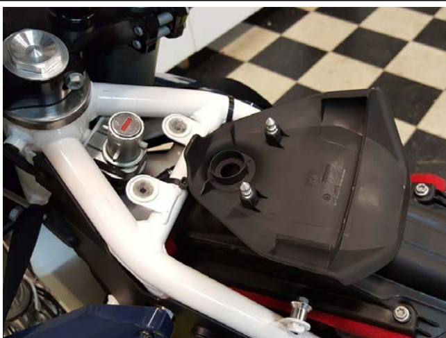
Remove the seat and ignition key cover
