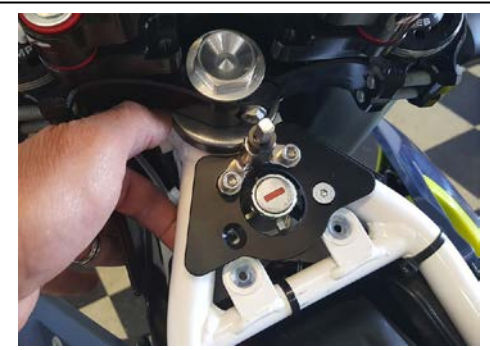
Once centered and "hooks" are on the frame, tighten the bolts using Loc-tite
