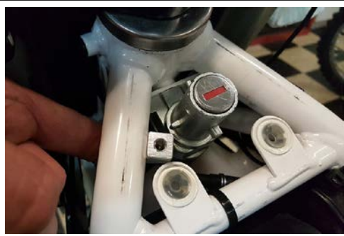
Insert the "hook" portion of the frame bracket around the contour of the frame
