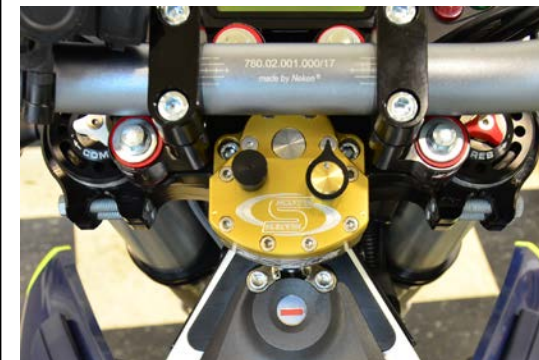
Cut the plastic ignition cover to suit your preference where it meets the tower.
