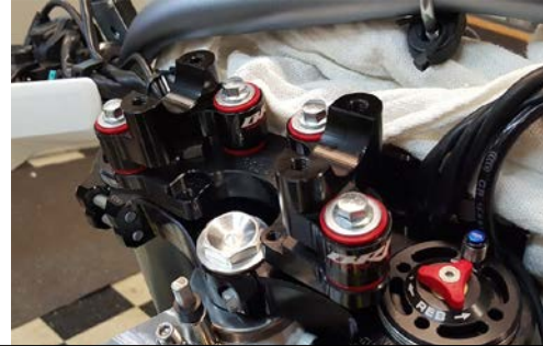
Install the Bar mounts to the base plate using the additional instruction sheet provided regarding the SUB mount itself.
