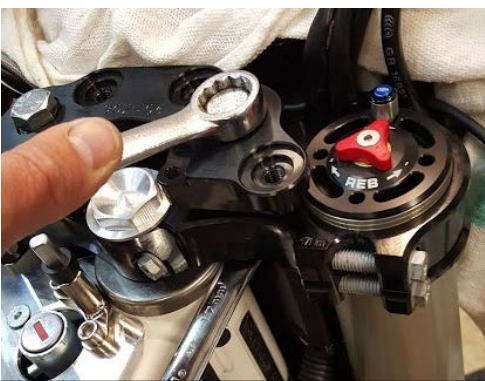
Tighten the Sub base plate to 36-38 ft lbs.
