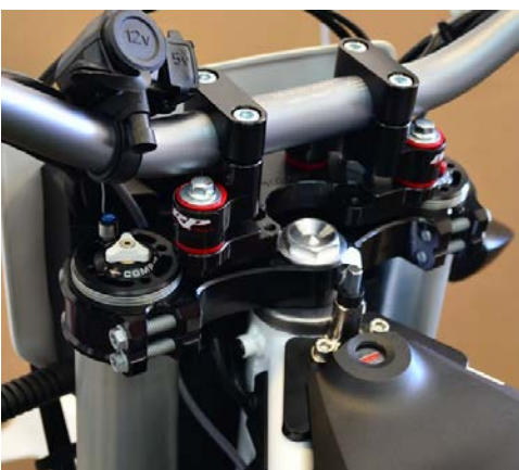
Cut the stock plastic ignition cover to match the contour of the frame bracket to suit your preference. Use 400grit sandpaper to make the edges smooth
