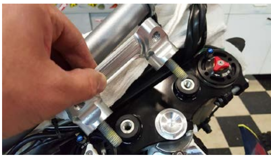
Remove the stock upper bar mounts 1st, then lay the bars forward of the triple clamp in a towel. Remove the lower handlebar mount and the stock-lower-rubber-mounts from the triple clamp.
