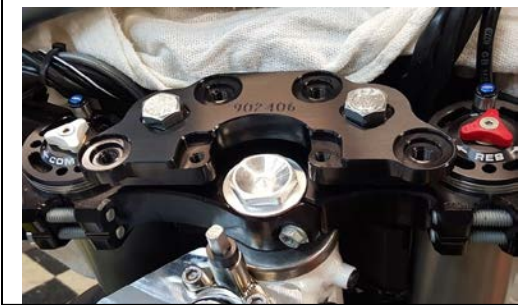
Install the SUB mount base plate to the triple clamp using the 12x60 bolts supplied, then new aluminum cones on the bottom with washers and locking nuts to 36-38ft
