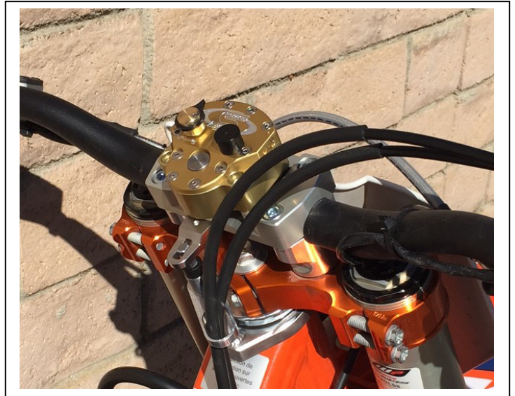
Be sure when using the stock lower cradle that you tighten the high side bolts first. In the reversed position the high side would be toward the rear of the bike.
