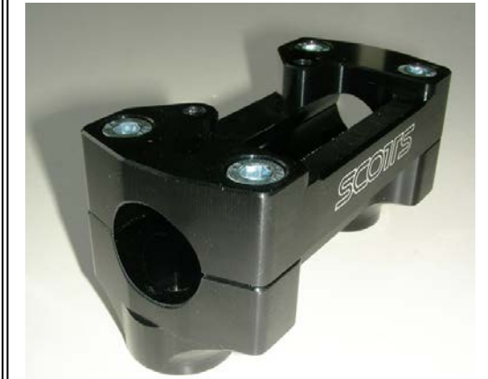
This shows the new one piece HD Scotts lower cradle and Barclamp to replace the rather weak stock unit that bends easily with simple tip overs.
