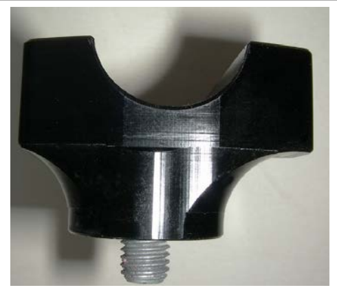
Shown here is the lower Barclamp cradle with the bars in the Forward position, notice the center line of bars are forward of the center line of the bolt out the bottom.
