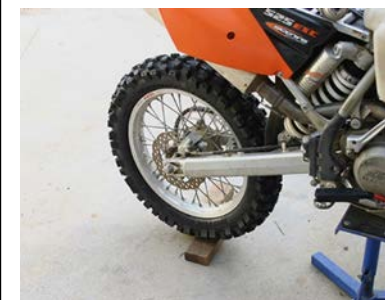
Block the rear wheel also, pushing pressure on the front end to hold the forks tightly in place.
