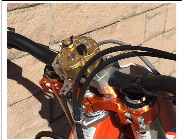
Shown here is the lower Barclamp cradle with the bars in the Rearward position, notice the center line of bars are rearward of the center line of the bolt
