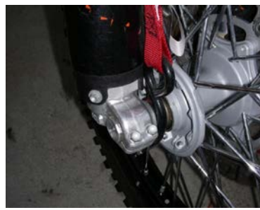
Run a tie down from the front axle up and over the backbone to the other side axle.
