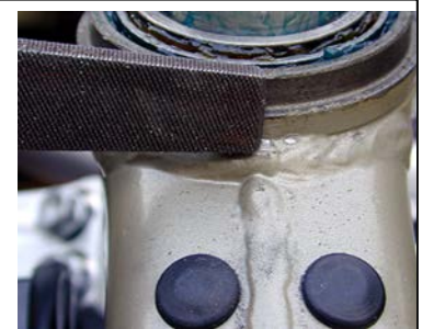
Using a sharp file, start at the high spots and trial fit the bracket until it fits.
