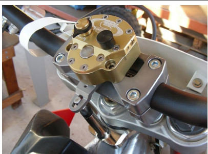
Shown here is the oversized bar conversion kit which eliminates the cross bar altogether and allows mounting in either reversed or standard position.
