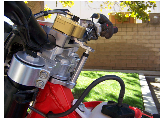
File welds keeping the frame bracket from clamping tightly around head tube
