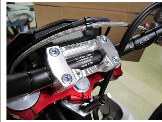
Frame bracket down far enough so the bearing shroud does not make contact with the bracket
