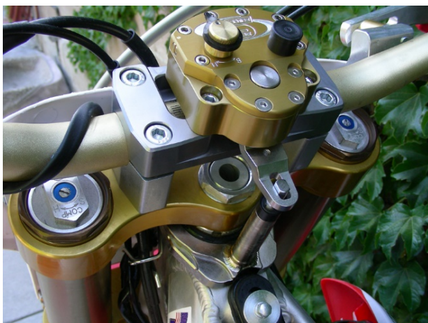
Finished kit installed using the stock handlebars with the stabilizer in the “reversed” position
