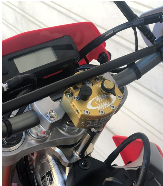
Finished kit installed using the stock handlebars with the stabilizer in the “reversed” position
