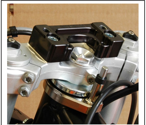
Bolt the SUB mount to the triple clamp, Using the Allen bolts provided.
