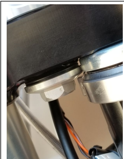
This picture shows the bolt rotated so the flat of the bolt head gives more clearance to the frame bracket.
