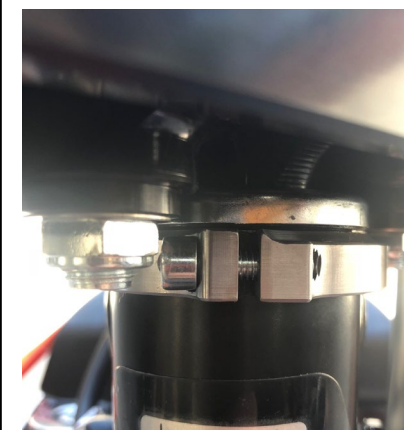
This shows the pinch bolt area with proper clearance to the bolt head at full lock.
