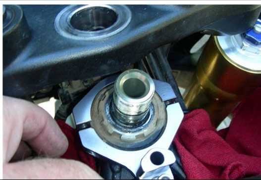
Lift the triple clamp up just high enough to install the new frame bracket. (Frame bracket shown may not be identical to yours).
