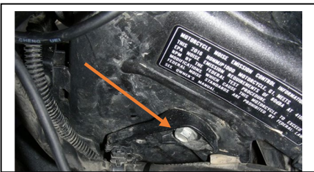
Remove any cable mounts and guides like shown, to give the cables more room to remove triple clamp.
