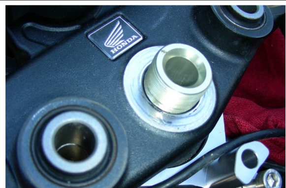
Remove the 30mm nut holding your triple clamp tight to the steering tube.
