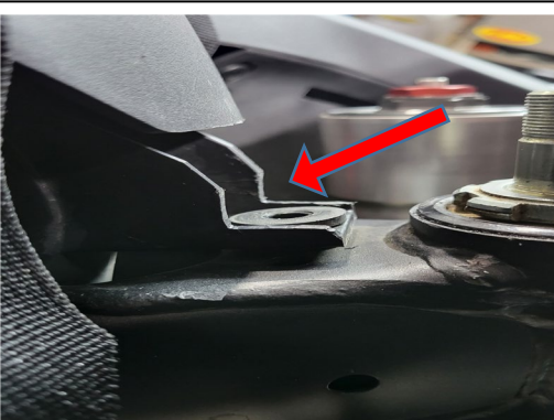
Once the forward tab is filed or ground for clearance it will look like this.
