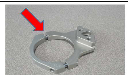
Start the frame bracket bolts so the gap is 4mm or so, to allow for easier installation later.
