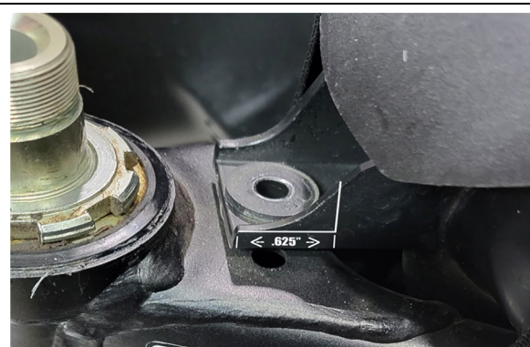
Modify the front tab mount tab by filing the area marked in white. We used a Dremel drum sanding roll but any appropriate tool to reach the goal is ok.
