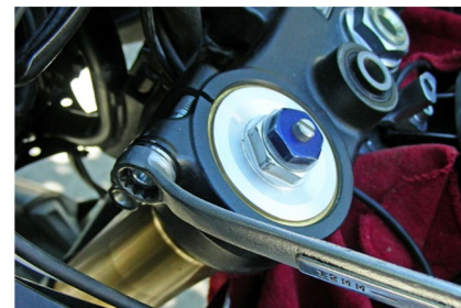
Loosen the fork pinch bolts. Remove one completely to remind you later to tighten them back up.
