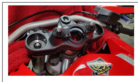
Step #12 Install the Scotts base plate over the studs so the recess on the plate matches the flange on the stud.
