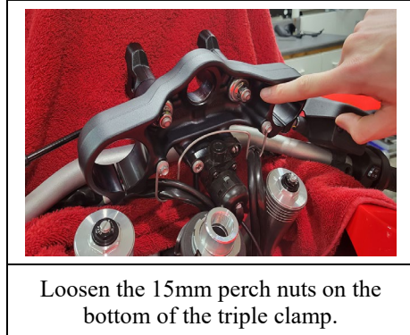
Remove handlebars and lay forward in a towel or protective blanket
