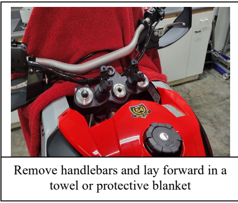
Remove upper triple clamp pinch bolts & put one aside for a reminder they're loose
