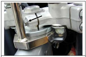
Where to file pinch the bolt area, if necessary. And nut to frame bracket clearance when done.
