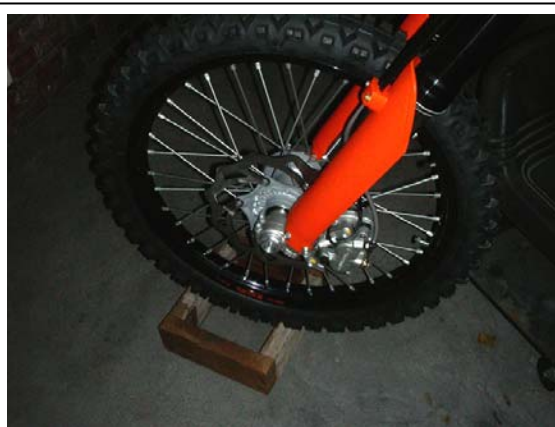
Block front & rear wheel to keep forks up and tight
