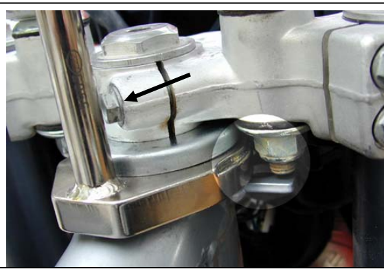
Where to file pinch the bolt area, if necessary. And nut to frame bracket clearance when done.
