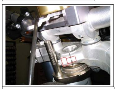
This shows where the bolt will approximately need to be after counter boring the pinch bolt hole deeper.
