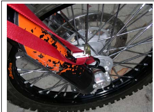
Hook tie down around axle up and over frame
