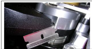
Keeping the TC mount straight while tightening.
