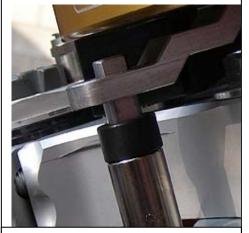
Tower Pin correct height after welding.
