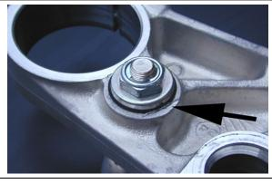
Photo at left shows the occasional mod required to some triple clamps in order to clear frame bracket.
