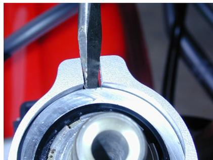
Remove bolt & spread gently to install
