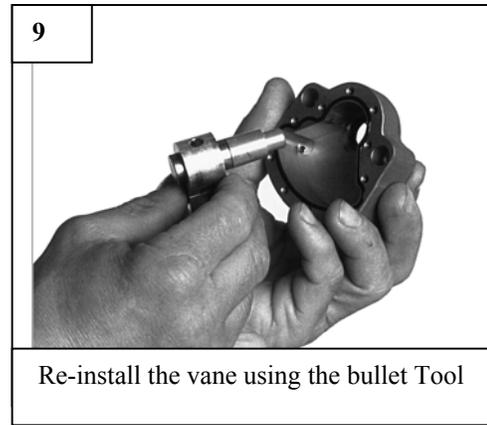
Re-install the vane using the bullet Tool
