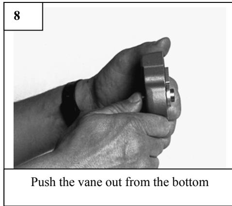
Push the vane out from the bottom
