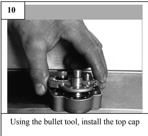
Using the bullet tool, install the top cap
