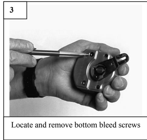
Locate and remove bottom bleed screws
