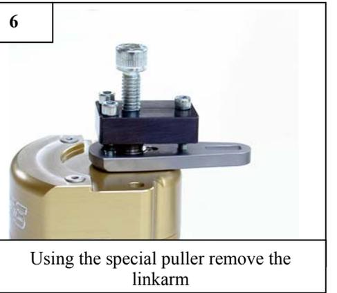
Using the special puller remove the linkarm
