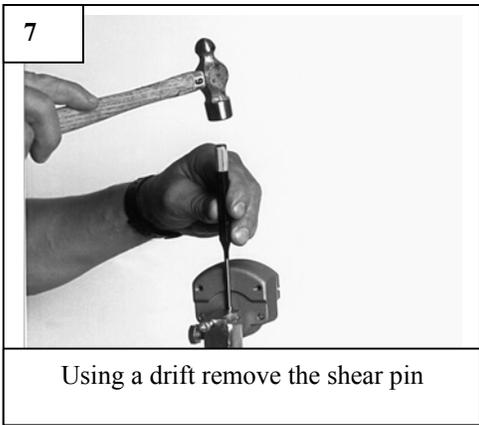
Using a drift remove the shear pin
