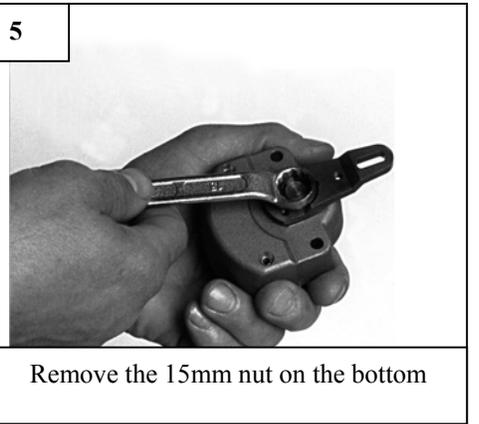
Remove the 15mm nut on the bottom
