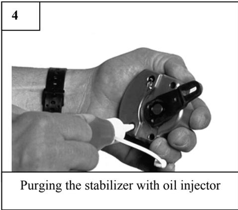
Purging the stabilizer with oil injector
