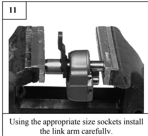
Using the appropriate size sockets install the link arm carefully.
