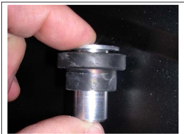
Install our new tank bushing through the stock rubber
