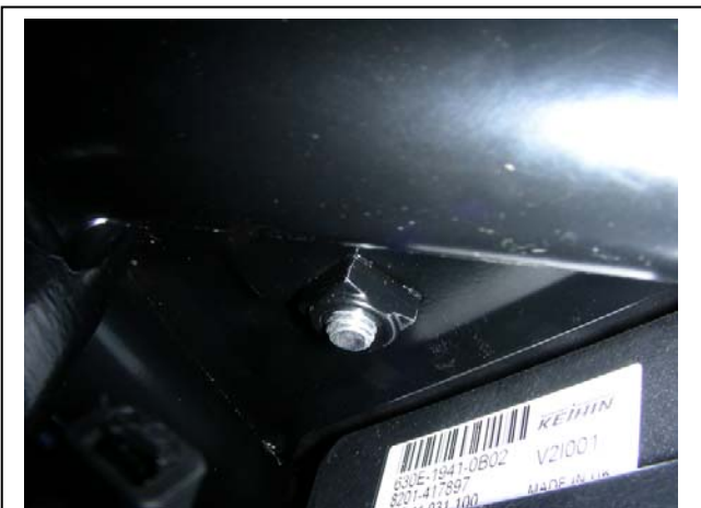
Nut located under the frame that tank bolt goes into. Our washer (at right) goes over it this nut after the bolt is tight. An additional nut is supplied for our washer.
