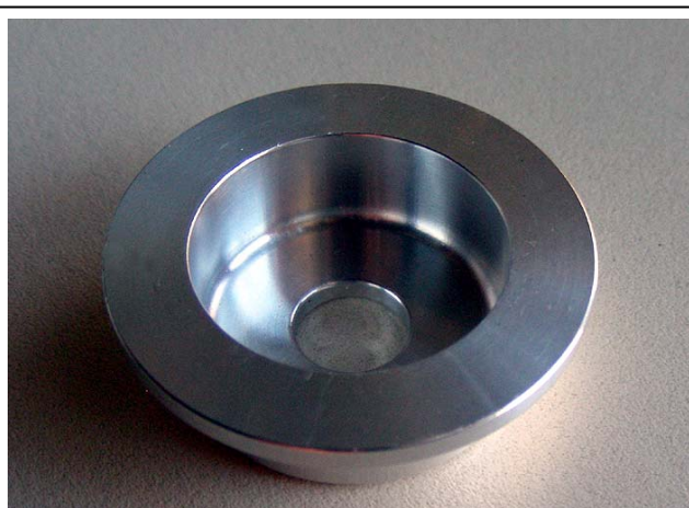
This bushing goes over the one shown at left after you've tightened the tank bolt completely. This washer adds a larger footprint to securing the frame bracket to frame.
