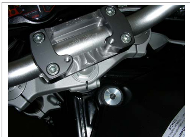
Barclamp and tank bushing installed
