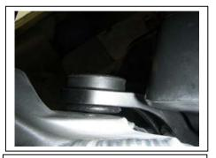
250 ONLY: you must invert the stock Tank bushing so the thin side is down And install 3mm washer under tab.
