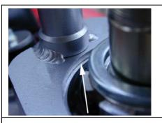
Be sure the frame bracket is <u>all the</u> <u>way down</u> flush with the head tube, all the way around the entire surface.
