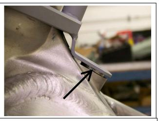
Use the washers provided to space the tab correctly. Usually one below and one above is most common.
