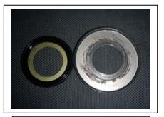
07 Seal on the left. 08 seal on the right. Must use 07 style seal with our kit to allow frame bracket to fit.
