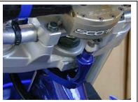
Shown above are the Scotts Billet Triple clamp with Protaper bars. These require no modifications and bolt right on.
