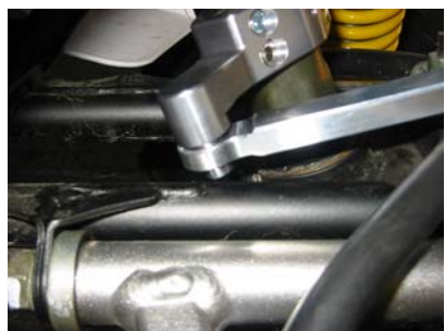
Be sure the Allen bolt clears the frame
