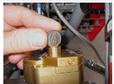
Adjusting the high speed with a dime
