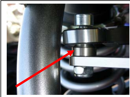
Stainless spacer between link arm & strut
