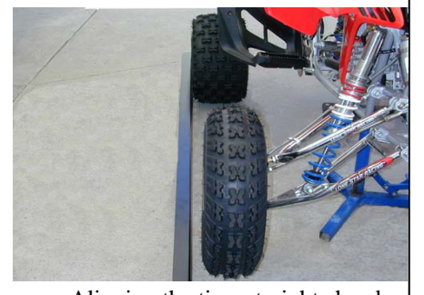
Aligning the tires straight ahead
