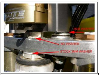
450's: install (1) washer between the sub mount and rubber cone on each side of the sub mount.
