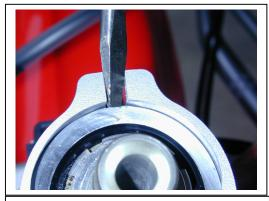
Spread the bracket gently, only enough to allow it to slide over the head tube.
