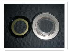
Our Seal on the left. stock seal on the right. Must use our style seal with our kit to allow frame bracket to fit.
