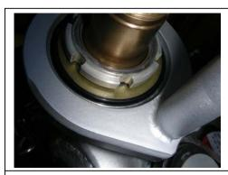
The frame bracket must down flush, all the way around on the top of the head tube.
