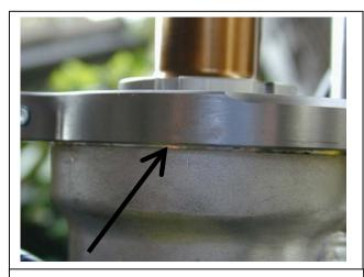
Once the frame bracket is on, the machined area showing below the bracket should be equally spaced.
