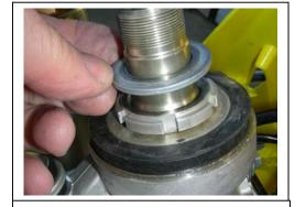
Put the stem spacer here on top of jam nut
