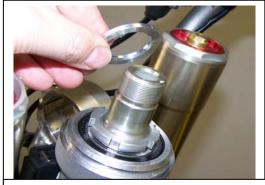
Install the provided stem washer on top of the jam nut, and under the triple clamp
