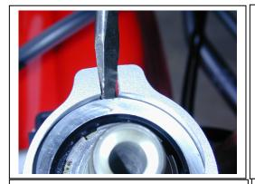
Spread the bracket gently, only enough to allow it to slide over the head tube.
