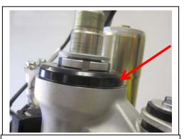
Remove the black dust cover shown here. The stock head bearing is a sealed bearing does not require this additional dust cover.
