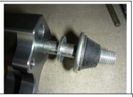
450: install the 2mm washers between the cone and bottom of the sub mount
