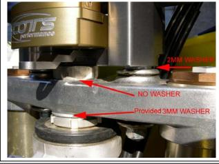
450's: install the washer detail as show above to obtain the correct spacing for linkarm to tower height.
