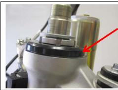
Remove the black dust cover shown here. The stock head bearing is a sealed bearing does not require this additional dust cover.
