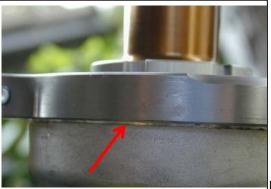
The machined area showing below the bracket should be equally spaced to be sure it's flush.
