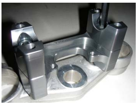
Next bolt the lower perches to the base
