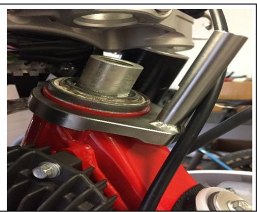
Keep the frame bracket low enough so when the shroud is on, no contact to the bracket.
