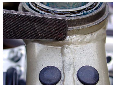
Using a sharp file, file away any slag that will prevent the frame bracket from fitting tightly around the head tube.
