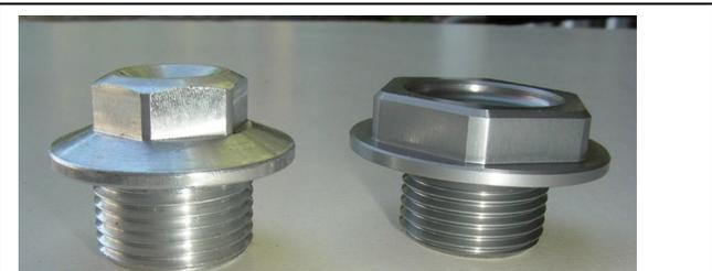
The stock 2015 stem nut shown at left.... Use Scotts Replacement nut @ right for 2015-on rubber SUBS
