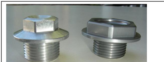
The stock 2015 stem nut shown at left.... Use Scotts Replacement nut shown @ right for 2015-on rubber SUBs
