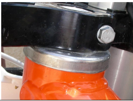
Stock frame welds may need some filing
