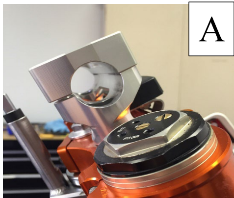
Shown here is the lower Barclamp cradle with the bars in the Forward position. You must tighten the front bolts first, so the Barclamp butts down tightly.
