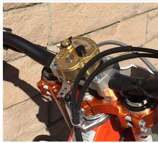
This shows the tower pin centered in the middle of the slot of the link arm. If yours is not centered you may have the lower perches reversed and need to correct the problem or you could damage your stabilizer internally.
