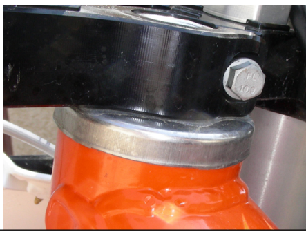
Stock frame welds may need some filing
