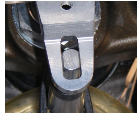
This shows the tower pin centered in the middle of the slot of the link arm. If yours is not centered you may have the lower perches reversed and need to correct the problem or you could damage your stabilizer internally.
