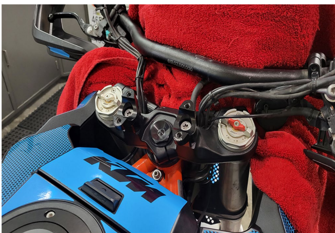
Remove upper bar mounts / lay bars forward out of the way
