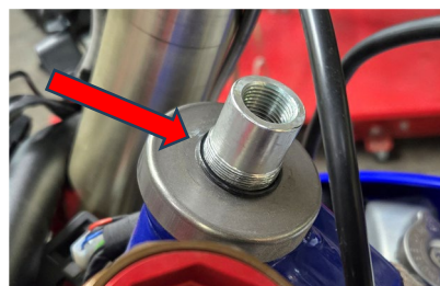
Note the o-ring on top of the stock dust cover. The O-ring gets re-used.
