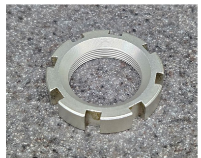
Note the chamfer faces down so the the O-ring fits inside the chamfer.
