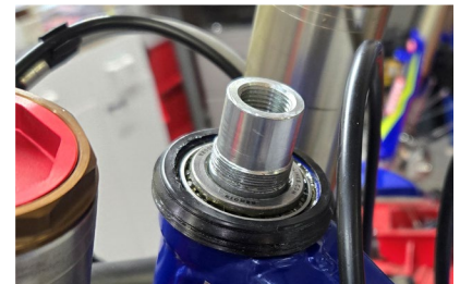
Remove the stock dust cover exposing the stock head tube seal.
