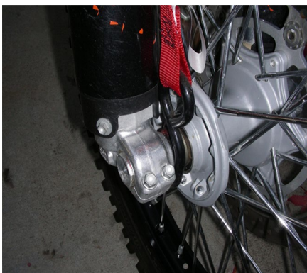
Tie the front wheel up with a tie down over the backbone of the frame, hook one end on the front axle and the other end on the brake caliper on other side.
