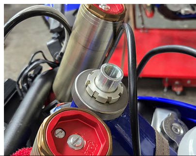
Remove the top triple clamp exposing the castle nut & dust cover
