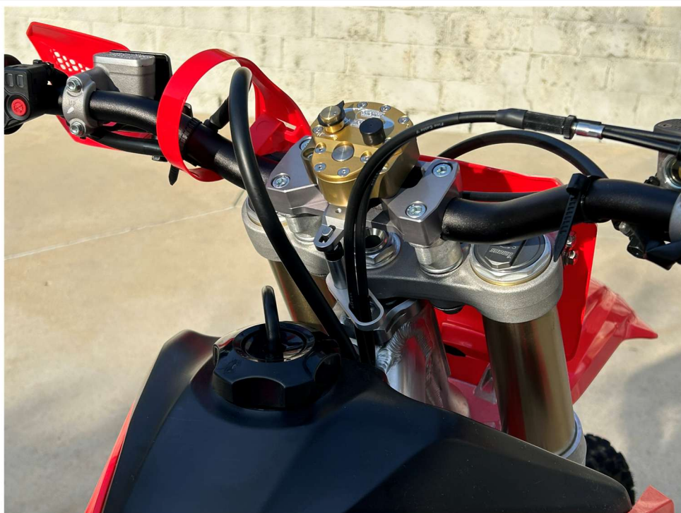
Finished kit installed using the stock oversized handlebars and optional Clean Speed cable guide
