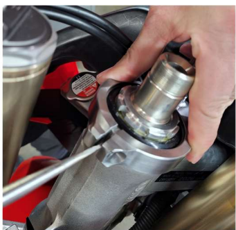
Remove bolt & spread bracket to install
