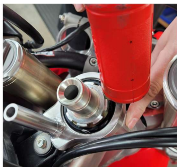
Tap bracket down until securely flush
